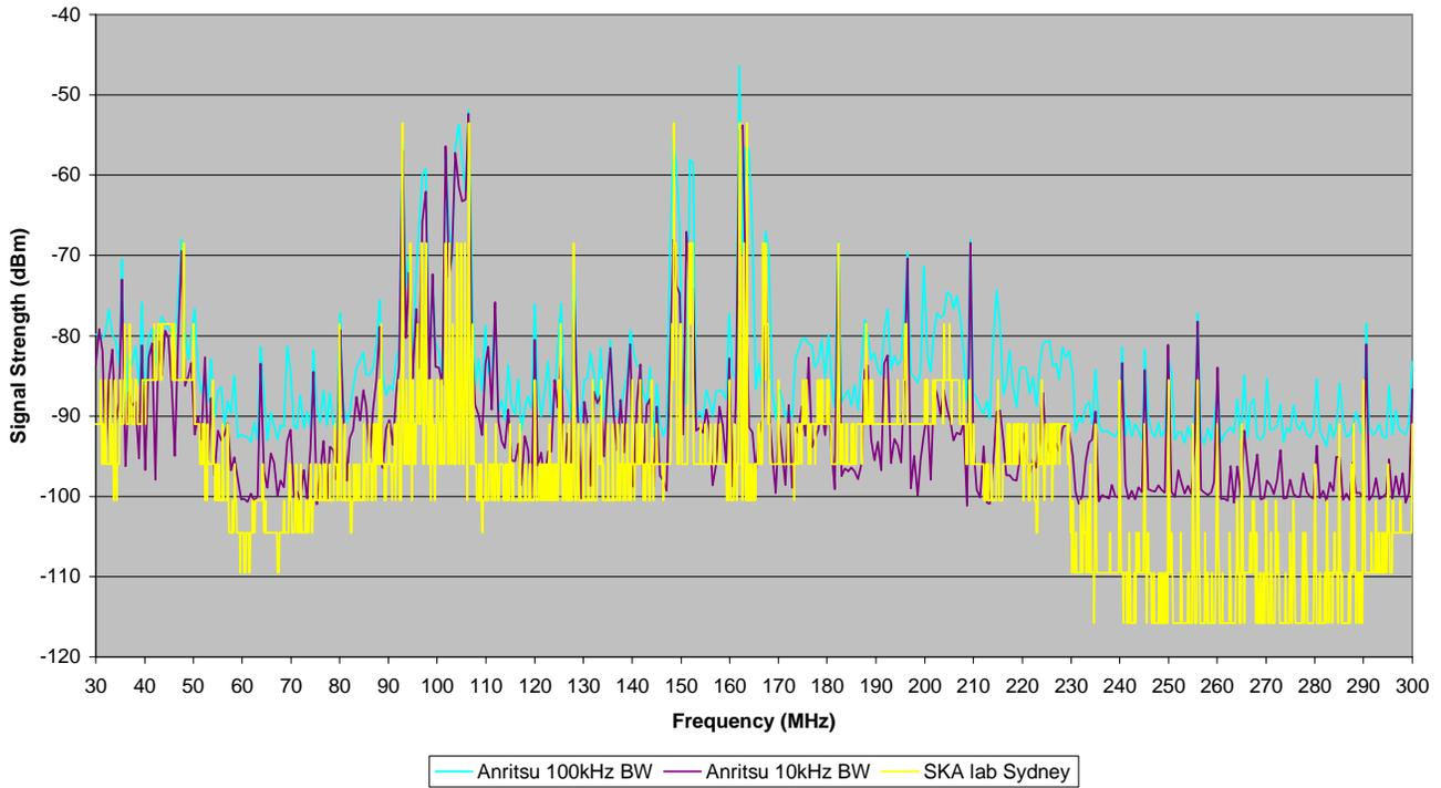
**Figure 20:** AR3000A WFM mode results for SKA lab converted to dBm and Anritzu Spectrum Analyzer scans.
