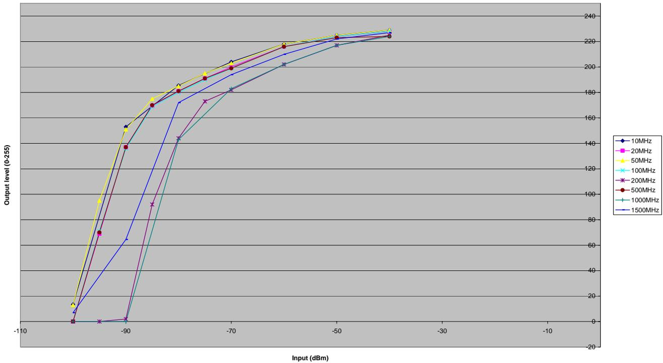
Figure 2: WR-1550e output level vs input amplitude for frequencies 10MHz to 1.5GHz in FMW.
