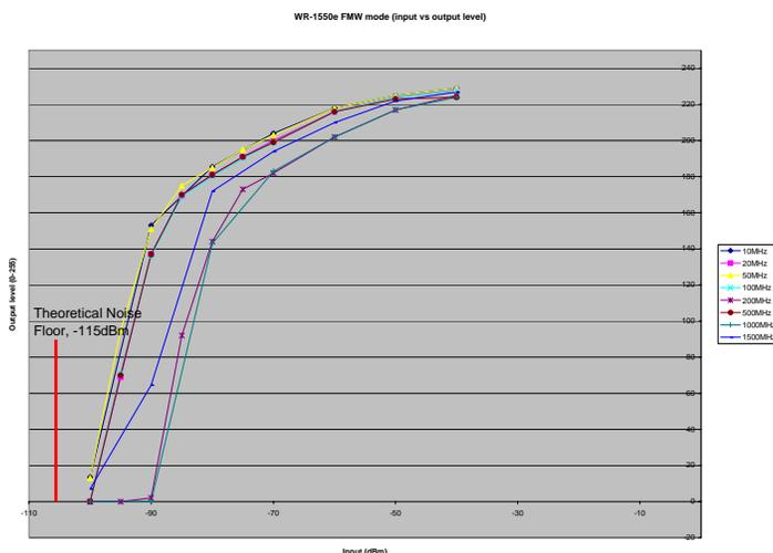
Figure 7: WR-1550e FMW theoretical noise floor.
