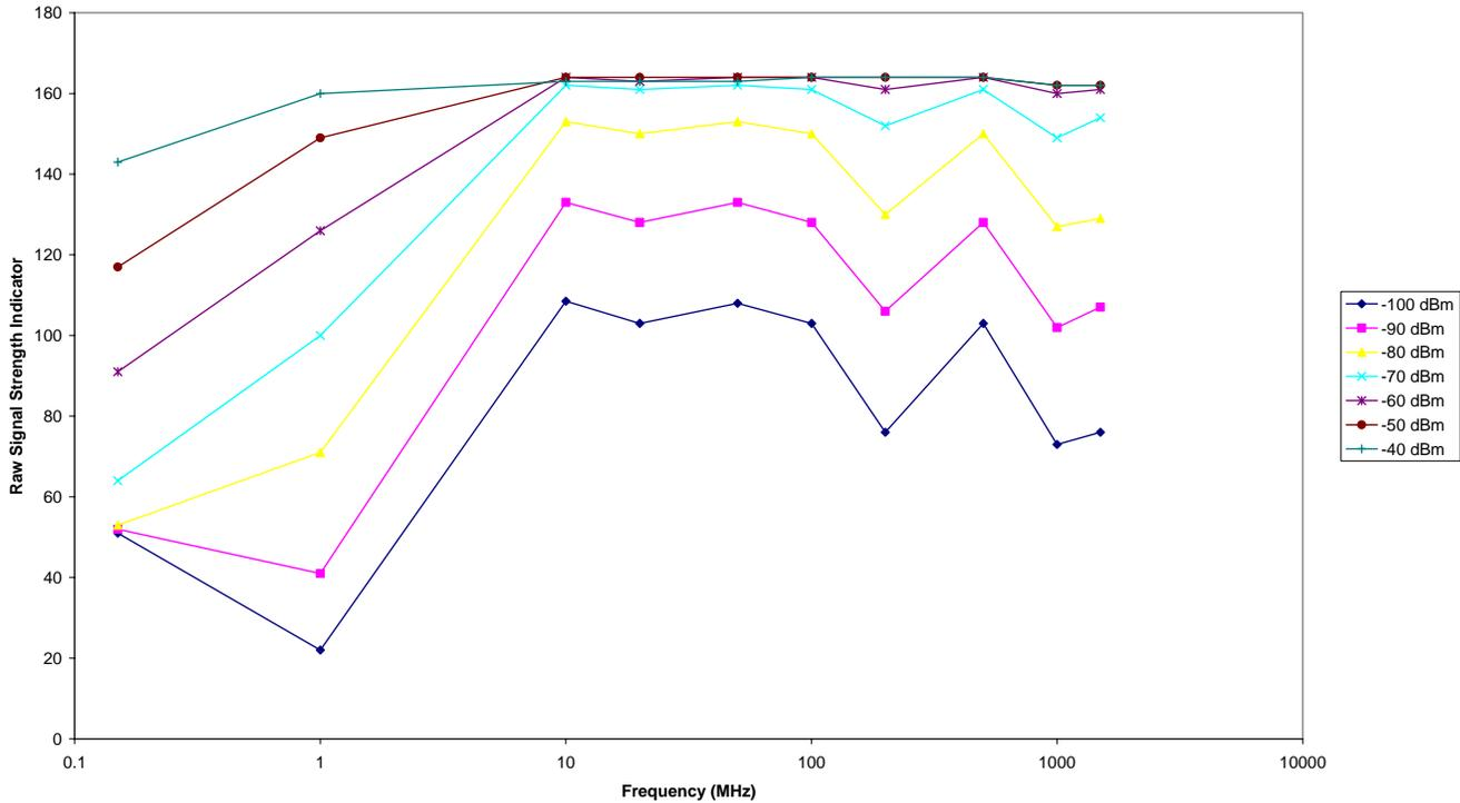
Figure 1: WR-1550e output level vs frequency for FMN.
