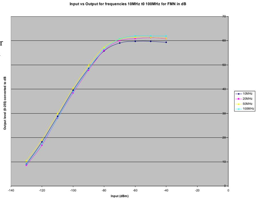
Figure 14: WR-1550e input level vs output level converted to dB for low frequencies.
