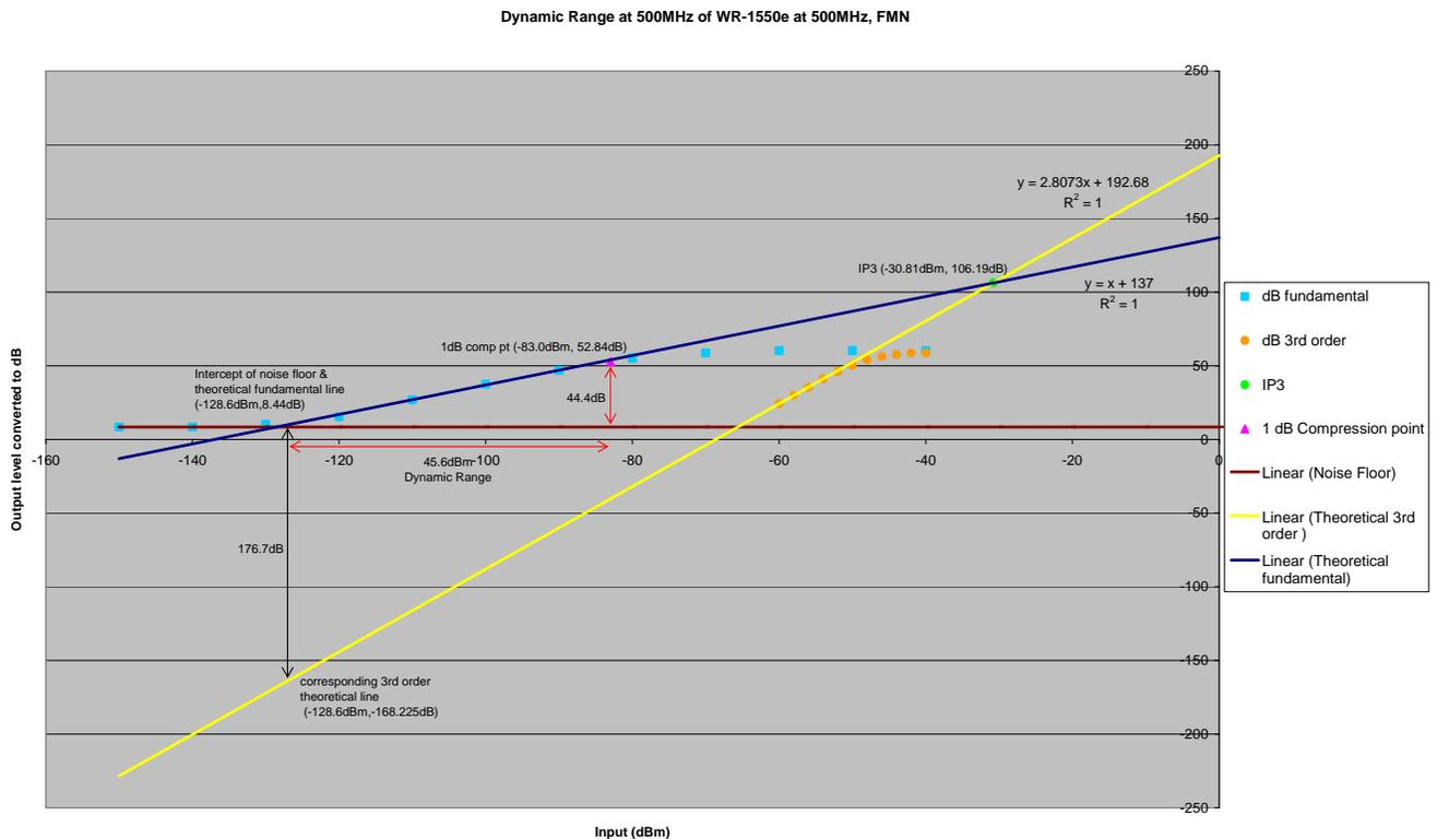
Figure 4: WR-1550e FMN Dynamic Range at 500MHz.
