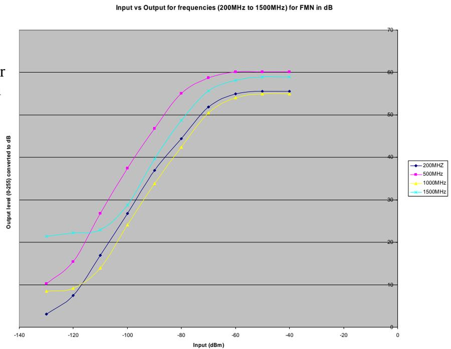
Figure 15: WR-1550e input level vs output level converted to dB for high frequencies.
