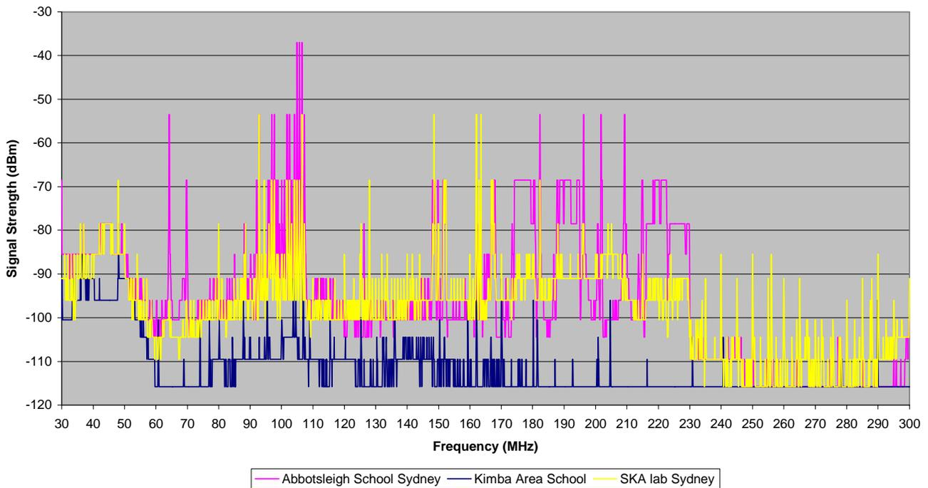
**Figure 19:** AR3000A WFM mode results from Kimba Area School, Abbotsleigh High School and SKA lab converted to dBm.
