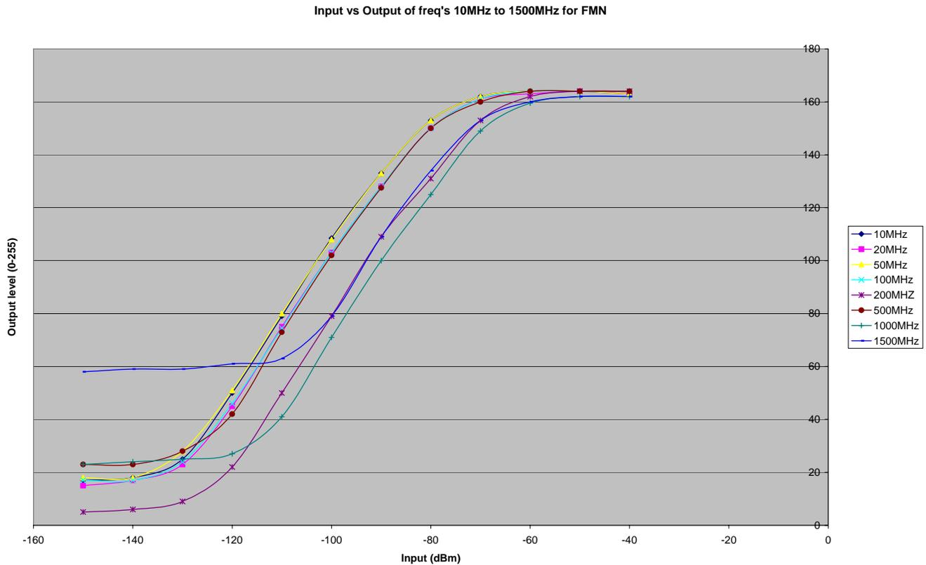
Figure 3: WR-1550e input level vs output level.
