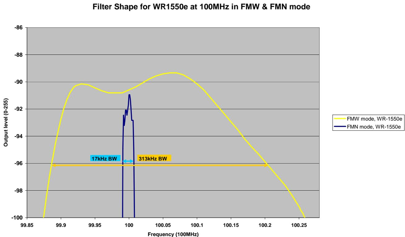
Figure 5: WR-1550e receiver selectivity at 100MHz for FMW & FMN.
