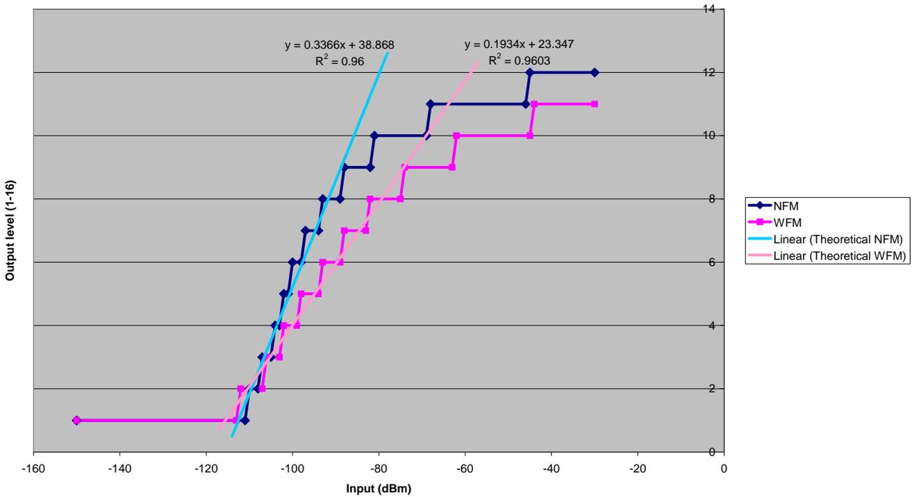
Figure 10: AR3000A output level for corresponding input amplitude in FMW & FMN mode.
