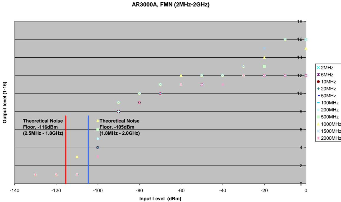
Figure 12: AR3000A theoretical noise floors for FMN mode.
