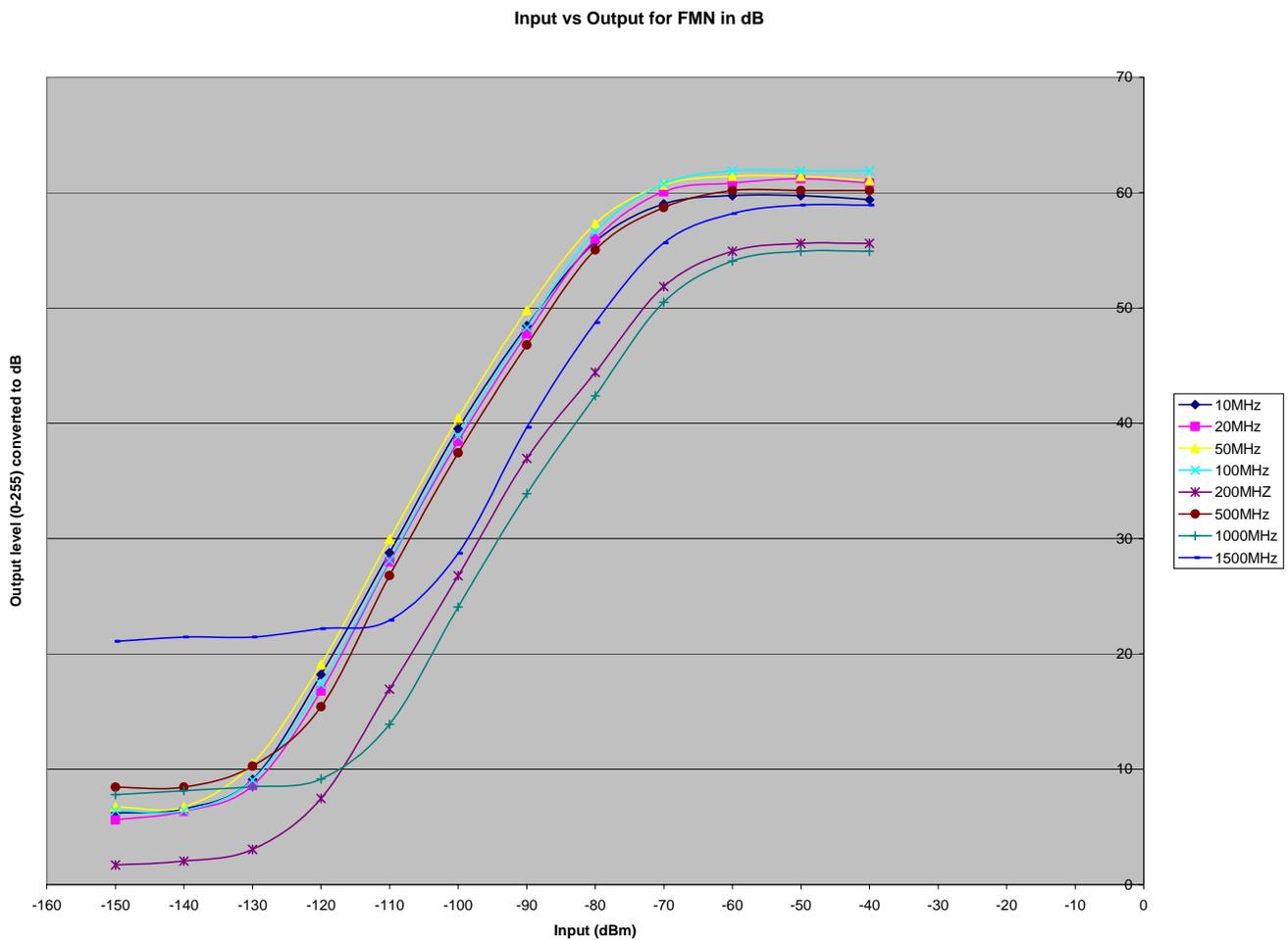
Figure 13: WR-1550e input level vs output level converted to dB.
