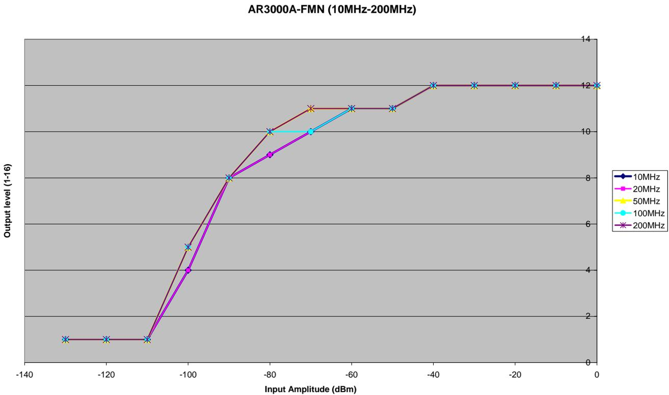
Figure 8: AR3000A output level vs input amplitude for frequencies 10MHz to 200MHz in FMN.
