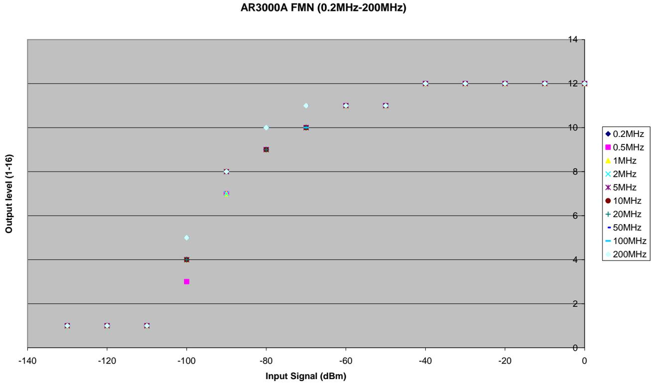
**Figure 16:** AR3000A output level vs input amplitude for frequencies 0.2MHz to 200MHz in FMN.
