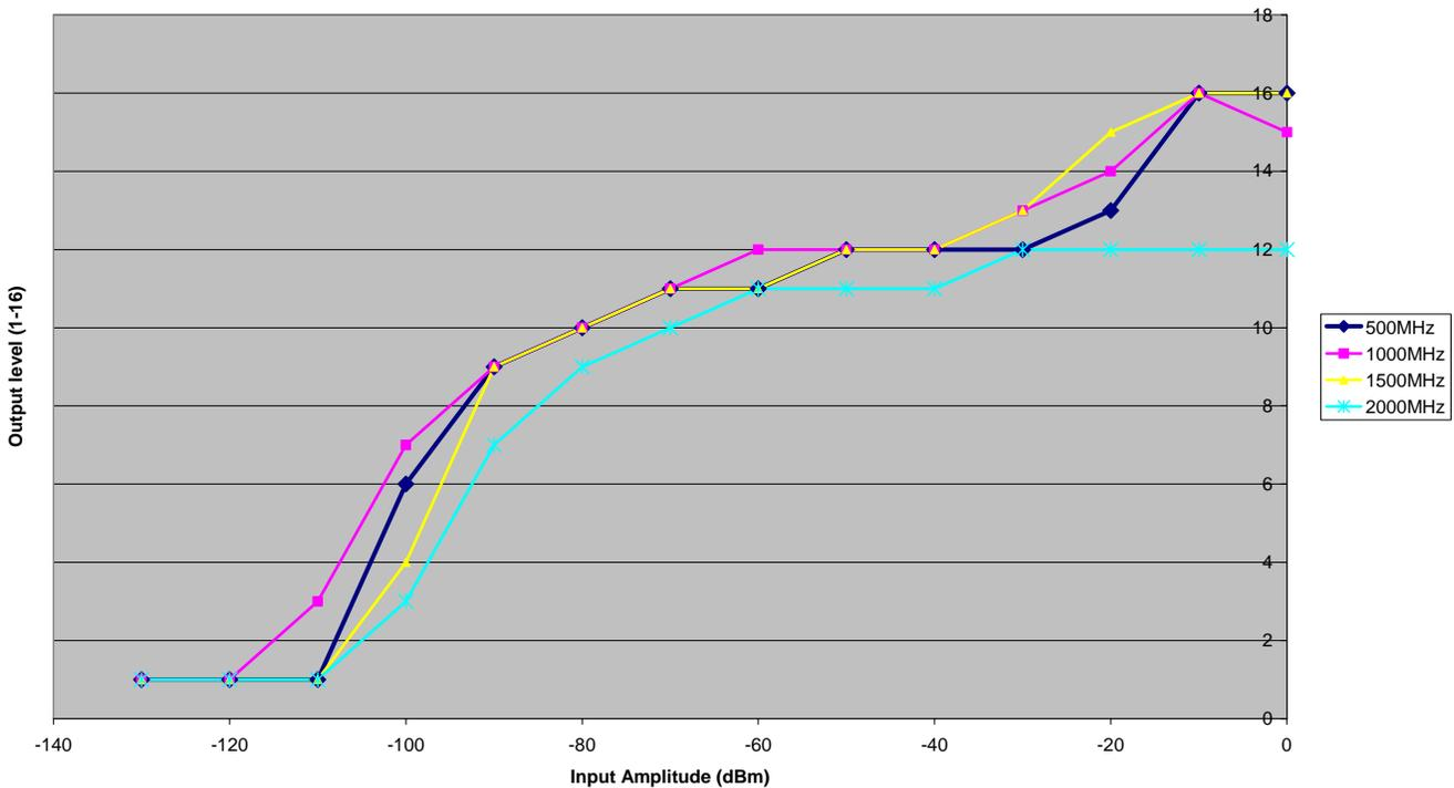
Figure 9: AR3000A output level vs input amplitude for frequencies 500MHz to 2GHz in FMN.
