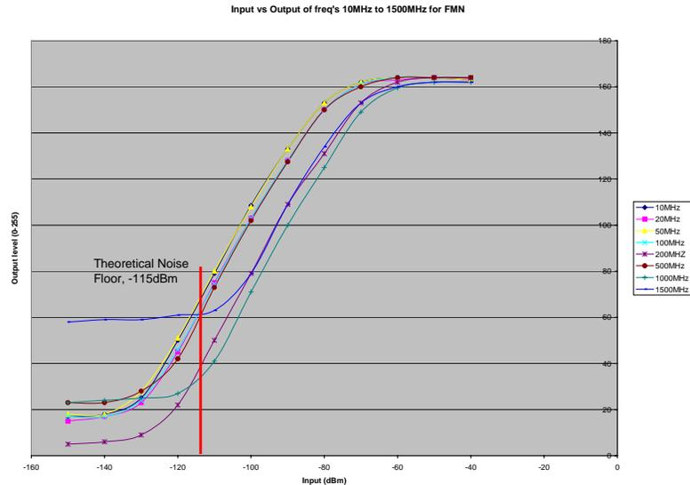
Figure 6: WR-1550e FMN theoretical noise floor.
