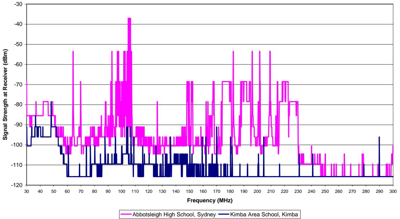
Figure 18: AR3000A WFM mode results from Kimba Area School and Abbotsleigh High School converted to dBm.
