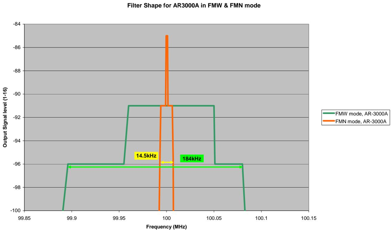
**Figure 11:** AR3000A receiver selectivity at 100MHz for FMW & FMN.
